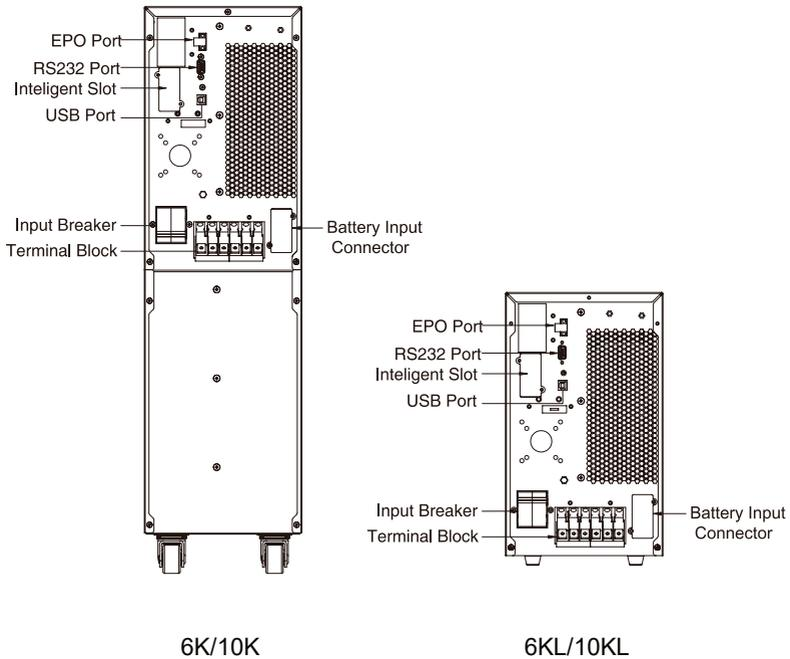
Fig.3-1 The rear view of 6K(L)/10K(L)
