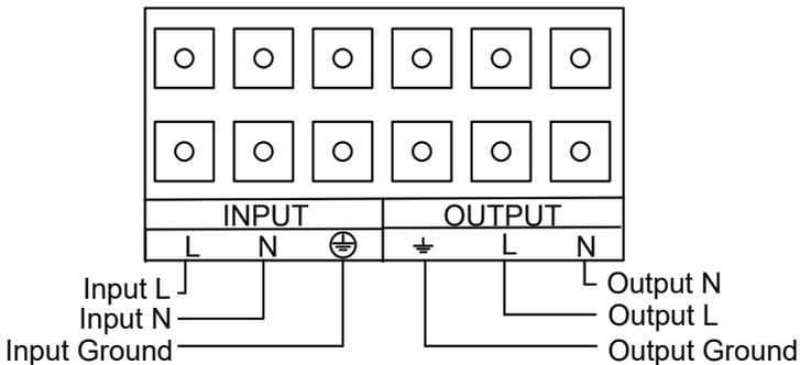
Fig.4-2 Input and output Terminal Block wiring diagram
